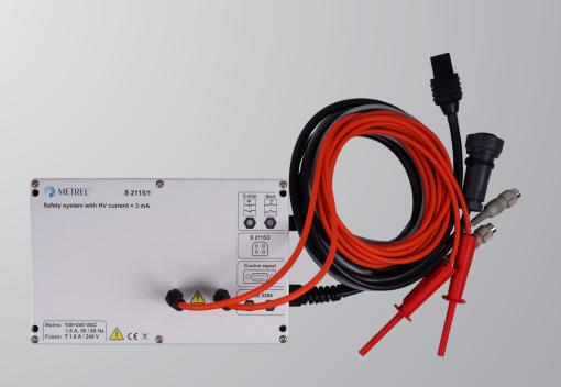
In many countries additional workplace safety measures are not needed during the high voltage testing with a.c. up to 3mA. If the current is higher than 3 mA a special test system with automatic protection against direct contact or a sealed off area with warning light and twohanded operation is required.
